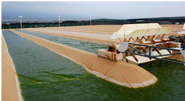
A demonstration plant for marine microalgae industrial cultivation in Kona, Hawaii, operated by Cellana LLC. Published in Greene et al (2016) Oceanography .
